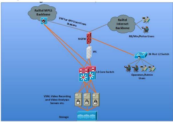
On top of this restricted and policy based access to all these users, there will be an additional IPS and advance malware protection layer. This additional IPS and advance malware protection layer of security will protect these systems for malicious activity, malware attacks and contamination from already compromised end points. Typical access and video traffic flow is shown on diagram given below:
