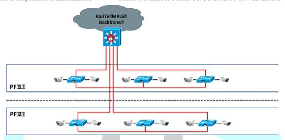
A separate VRF instance will be created on Type-IV Switch for different type of services (Surveillance, Wi-Fi etc). Access switches will separate these services in form of unique VLANs and maintain logical segregation between these services. This will maintain each service separately from traffic flow and QoS implementation perspective and improve network performance along with securing and isolating these services from each other.
