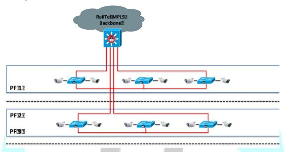
A separate VRF instance may be created on Type-IV switch for Railway Police Force users in addition to mentioned services in B type station. Railway Police Force users will have a secure client to for monitoring of stations through IP surveillance cameras.
