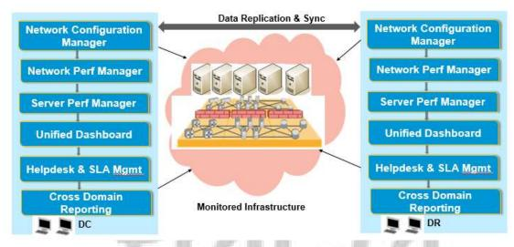
All the assets (pan-India) will be monitored through the central EMS deployed at one Data Center as a DC with the redundant infrastructure configured in other Data Center as a DR, in case of failover. There will be a continuous data replication & synchronization from DC to DR site on daily basis to prevent a loss of configuration changes in the event of losing the production instance.
