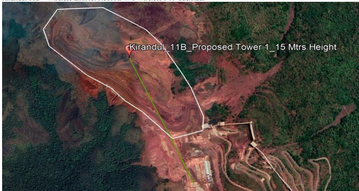
Fig 14 Kirandul 11B Wireless PTP Backhaul
