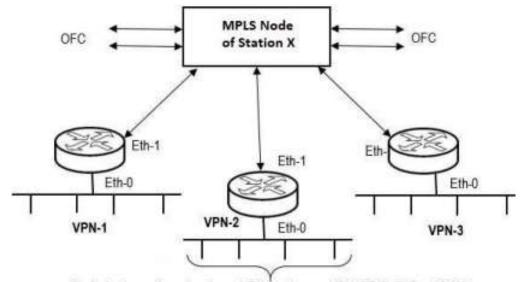
Typical scheme for extending a VPN service e.g UTN, FOIS, Railnet, CCTV etc at Stn X using small Edge router and its LAN connections for End points.
