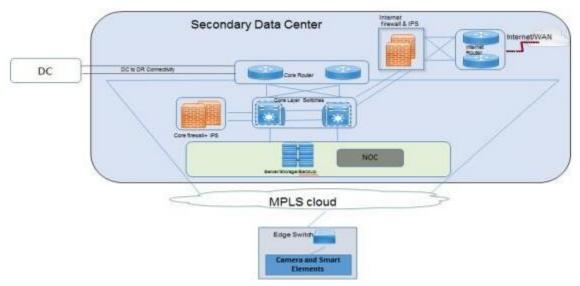
The DR Center is a minimalistic design to provide an operational continuity of Critical Smart City Utility applications in need of emergency. High level architecture of the DR remains like the DC.
