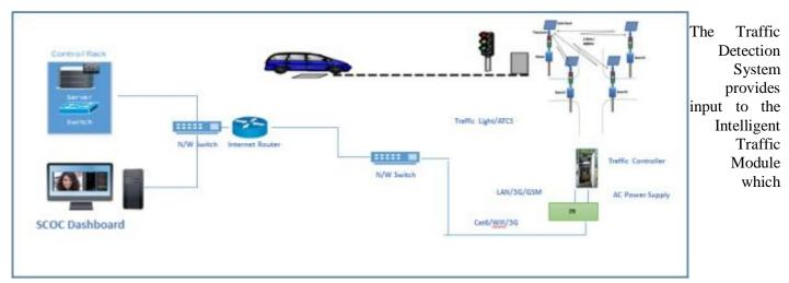
communicates with the Intelligent Traffic Control Server. The Intelligent Traffic Control Server runs the traffic control algorithm and provides input to the Intelligent Traffic Module which communicates with the Traffic Signal Controller to provide optimized traffic signal timing plans in a real-time scenario. The Surveillance System assists the city traffic operators monitor live operations at the city junctions and take corrective action if required.
