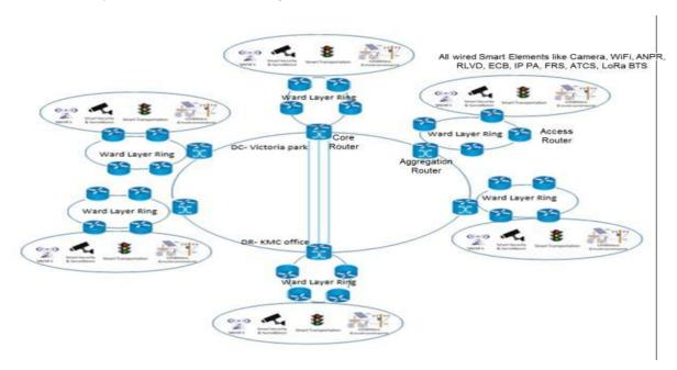
On a high level roughly 120 km of Optical fiber network is planned to cover the city backbone to connect the Smart elements and 50 Wards.
