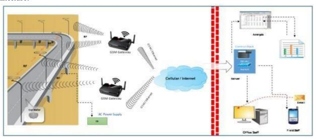
A typical streetlight monitoring and control system comprises of the following:
