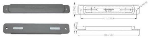
FM4000 tag is high performance radio frequency identification (RFID) tag designed especially for mount on metal or applications where environmental extremes or exposures are required. The F4000 tag can be applied using rivets, screws, or with a high bond strength acrylic adhesive, making it ideally suited for a broad range of applications where mount on metal or easy materials required.
