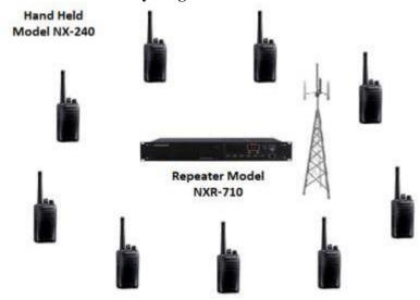
ICCC had Kenwood solution for the requirement. VHF Frequency to be programmed - Semi Duplex Tx / Rx frequency separation  $-\ 5$  MHz
