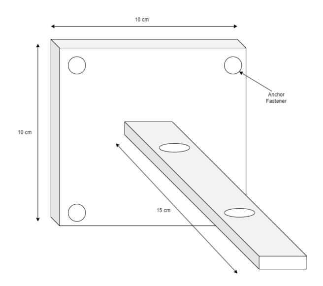
Material for Base Plate is MS and Sheet Thickness should not be less than 6 mm. For Arm itshould be MS angle size 1 inch.
